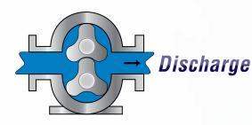
The fluid is transported around the channel by the rotor lobes, & is displaced as the rotor lobes re-mesh, generating pressure at the discharge port. Pump output is directly proportional to speed, and direction of flow is reversible.
