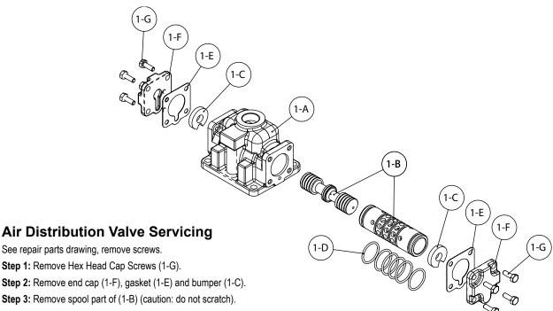
Step 2: Remove end cap (1-F), gasket (1-E) and bumper (1-C).
