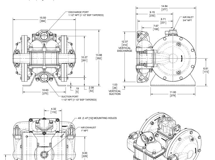
Model HDB1½-A features 1½" NPT threaded connections. Model HDB40-A features 11/2" BSP Tapered connections.
