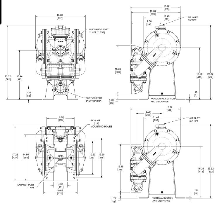
Model HDB2-A features 2" NPT threaded connections. Model HDB50-A features 2" BSP Tapered connections.
