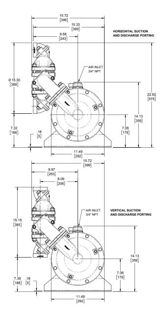
Model HDB2-A features 2" NPT threaded connections. Model HDB50-A features 2" BSP Tapered connections.
