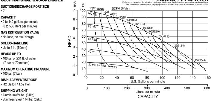
These pump models are designed to pump the following fluids: Crude Oil, Salt Water, Drilling Mud, Condensate, Lubrication Oils, Glycol, Caustic Liquids, and Acids."
