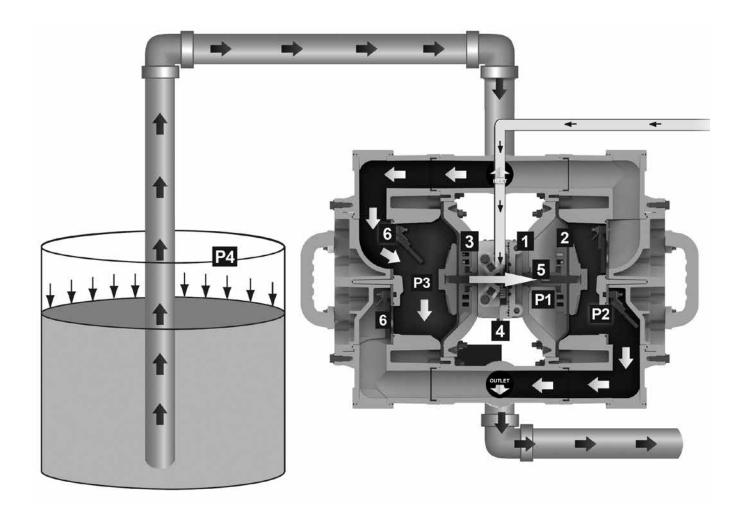
Gas-Operated Double Diaphragm (GODD) pumps are powered by compressed air or nitrogen.
