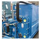
Screw pumps for the ship pump package:
