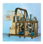
Pumps: L 20 with magnetic coupling. Pressure: approx. 12 bar. Viscosity: Polyol 2.000 mm³/s.
