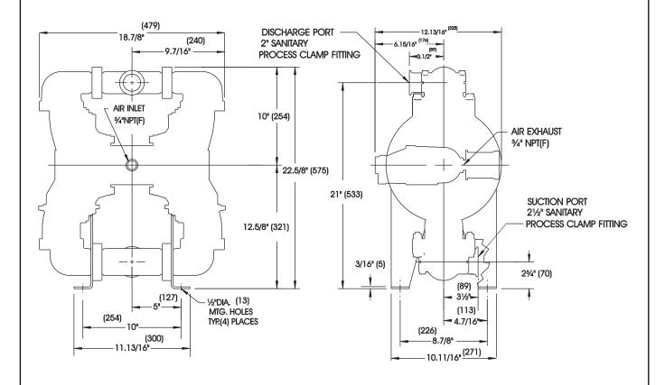
SUCTION 21/2" QUICK CONNECT SANITARY PROCESS CLAMP FITTINGS DISCHARGE 2" QUICK CONNECT SANITARY PROCESS CLAMP FITTINGS 34" NPT (F) AIR INLET PORT • 34" NPT (F) AIR EXHAUST PORT
