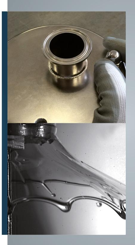
The Components of the PERA-PRINZ® Screw Pumps are machined with very accurate tolerances and with very high quality surface finishing, in order to reduce the clearance and minimize the leakages and backflow.
